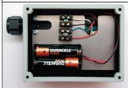
Figure C6b: Batteries in Piusi display w/ pulse out.
